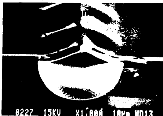
Fig. 2. Electronmicroscopic photograph of a cross section of a quartz wafer (with friendly approval of Industrial Microelectronics Center, Kista Sweden)
